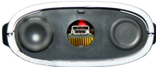
The service connector (UART interface) can be accessed without opening the enclosure after removing the protective red round cover.
